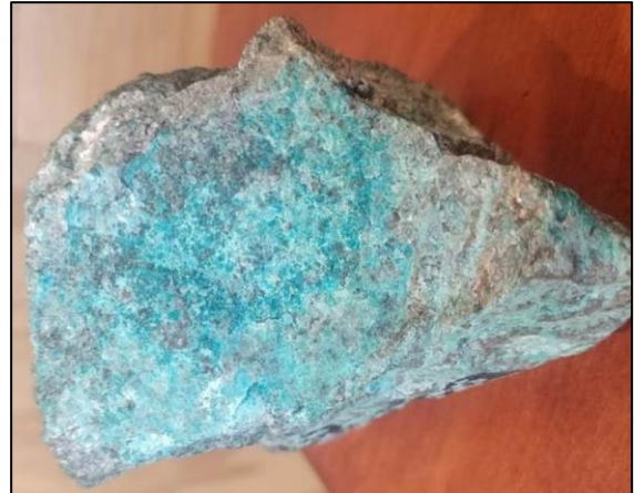
Figure 5. High grade 6% copper oxides as malachite, chrysocolla, and brochantite in silicified intrusive:
