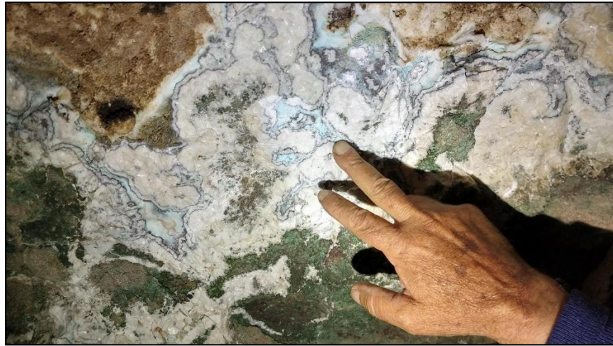
Figure 2. Banded silver sulphides, with barite, calcite and silica with characteristic green silver chloride oxides.
