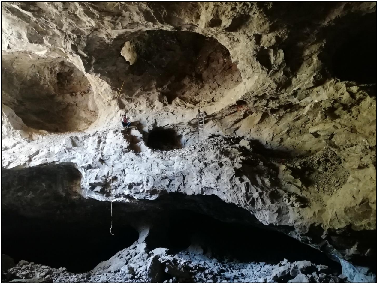
Figure 1. Historic silver mines at Plata Verde, an anastomosing sequence of silver mines, excavated in the late 1800's following silver mantos hosted within basaltic volcanics.
